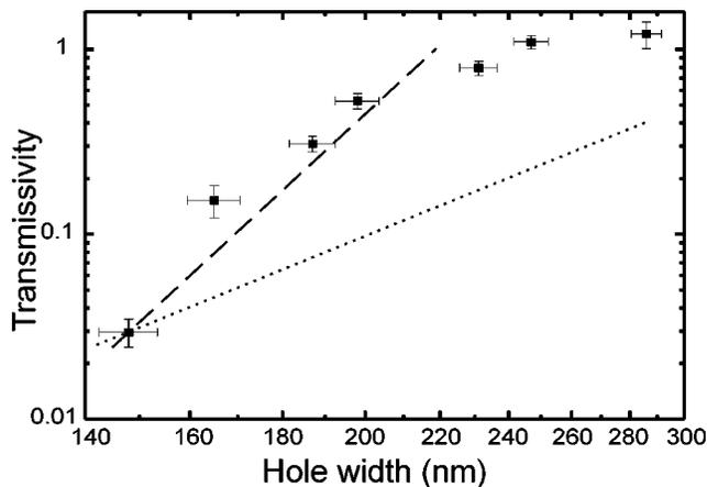
FIG. 3. The transmissivity as a function of hole width (double logarithmic scale, (1,0)-peak). The dotted line obeys  $T \propto d^4$ , the prediction according to the Bethe-Bouwkamp model. The dashed line obeys  $T \propto d^9$ . For small holes, the increase in transmissivity exceeds the  $d^4$  power law. For the largest holes the transmissivity saturates.
