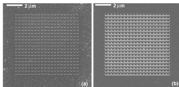
FIG. 1. Focused ion-beam images of two periodic arrays of square, subwavelength holes. Both structures are fabricated in a 200-nm-thick Au film and have a period of 425 nm. The hole width of the squares in (a) is 148 nm. In (b) the hole width is 286 nm. The square holes have sharp edges and are highly uniform.
