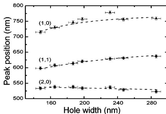
FIG. 4. The wavelength of the different peaks as function of hole width. For increasing hole width the (1,0)- and the (1,1)-peak shift to longer wavelengths, the (2,0)-peak shifts to smaller wavelengths for increasing hole width. The dashed lines are guides to the eye.
