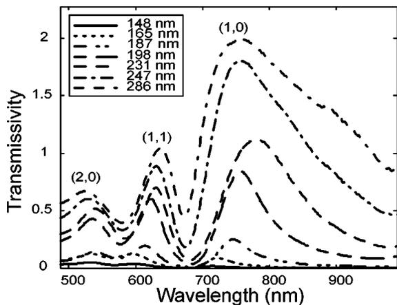
FIG. 2. The transmissivity as a function of wavelength for square hole arrays with different hole width. The legend lists the hole widths. The transmissivity increases and the peaks broaden for increasing hole width. The assignments of the three different groups of maxima is given by the numbers in brackets.
