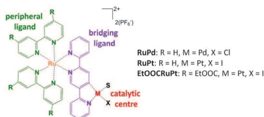
Fig. 1 Structure of the photocatalysts RuPd , RuPt and EtOOCRuPt . The ester unsubstituted and substituted precursors are denoted as Ru and EtOOCRu , respectively. S = solvent (acetonitrile). See Section S3, ESI† for more details.
