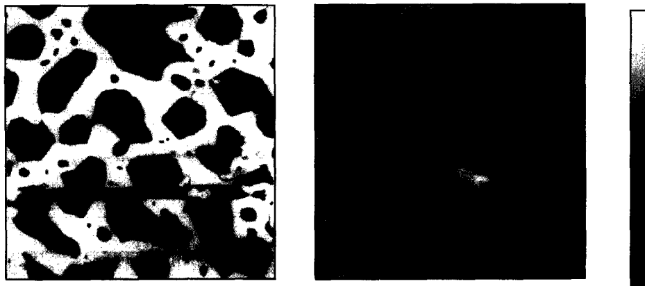
Fig. 4. Adhesion mode AFM image of a lignoceric acid Langmuir–Blodgett film. The dark areas in the topography image represent the holes in the LB film. Scan area 2 \times 2 \mu\text{m} ; (a) represents height (range 2 nm), (b) the adhesion force (range 30–60 nN). Acquisition rate: 1400 ms/line.
